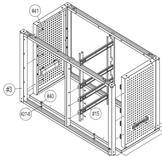
**Note:** Ensure all screws are fully tightened. Make sure the edges of all components are properly aligned before securing them.
