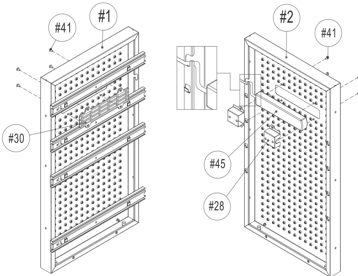
1. Attach (#45) USB multiple socket-outlet on the side panel, which can be assembled on (#1) the left side panel or (#2) the right side panel according to user demand.
