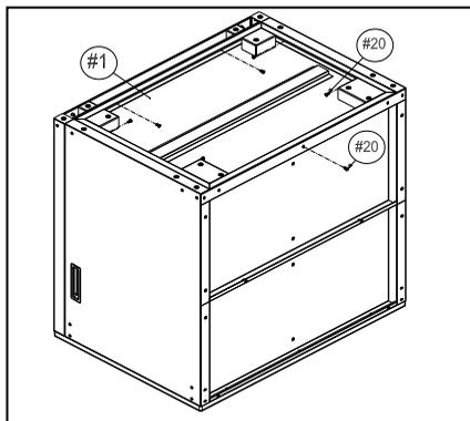
**Note:** Only the inner holes of the left side panel, right side panel, front frame and bottom back panel are used for attaching the bottom panel. The other four side holes at the corners are reserved for bumpers.
