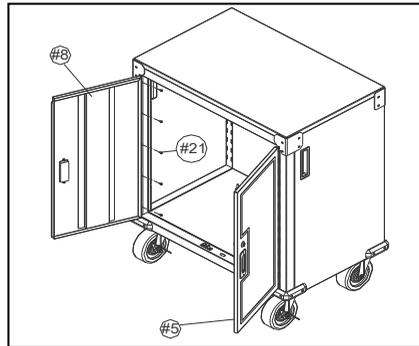
**Note:** The screw holes on the door hinge have some tolerance, thereby enabling the door to be adjusted and centred on the frame.
